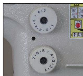
One touch switchover for two different stitch lengths (DS device)
